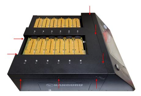
3. Remove the top panel and remove the 2x screws that attach the Source port board.
