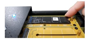
5. Slide the Locking Pin into the notch at the back of the SSD.
