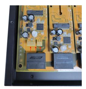
5. Replace the Source port baord with the SATA adapter board. Fasten the SATA adapter board using the two screws that were removed in step 3.
