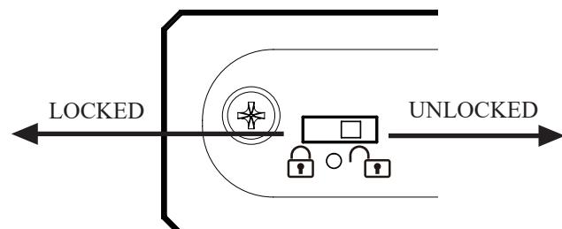
When set in the LOCKED position, the drive is write protected. When set in the UNLOCKED position, the drive is write enabled.
