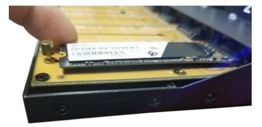
5. Slide the Drive Locking Pin into the notch located at the rear of the NVMe drive.
