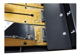
3. Insert the drive into one of the duplicator's M.2 ports at about a 30° angle. **Note:** you can identify the Source port location by the blue LED indicator.
