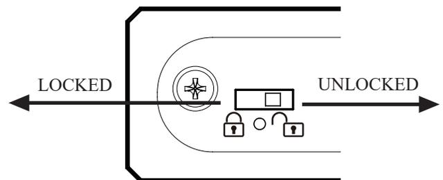
When set in the LOCKED position, the drive is write protected.
