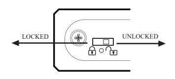
When set in the LOCKED position, the drive is write protected. When set in the UNLOCKED position, the drive is write enabled.
