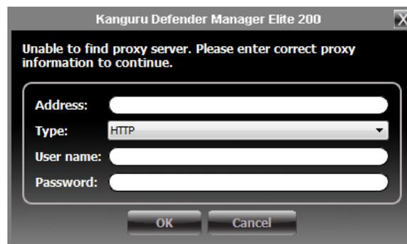
Enter the proxy address and the port to connect to in the address field (e.g. 192.168.0.193:8080 or proxycomp:8080). Select your proxy type and then enter your credentials. If KDMElite200 is able to connect to the proxy server using those credentials then the authentication information is saved in an encrypted proxy settings file.
