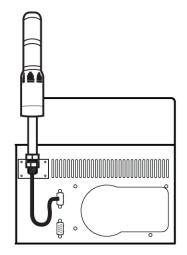
Congratulations! Your Light Tower is now mounted. While a duplication is in progress the Light Tower will blink green to indicate that it is working. When the duplication process has completed the Light Tower will show either a solid green or solid red light signifying a successful duplication or a failed duplication.
