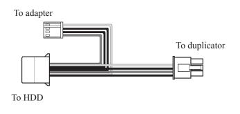
Complete connecting the cables as shown below.
