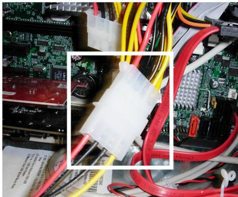
8. Connect the 15-pin SATA power connector to the Power Over eSATA bracket.
