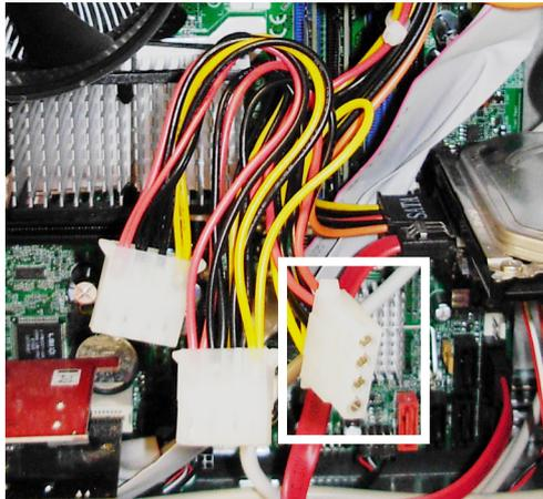
7. Connect the white end of the provided SATA power adapter cable to the computer's four-pin Molex power connector.
