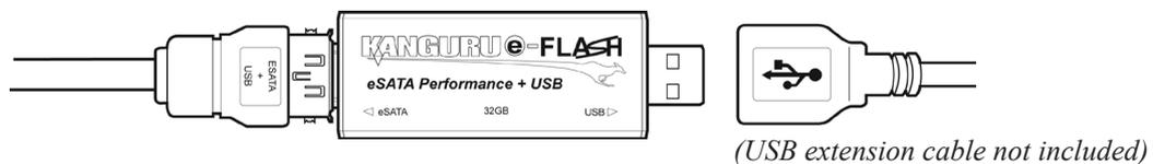
If you followed these steps and connected the device in the proper order, the eSATA connection will transfer data while the USB connection provides power.
