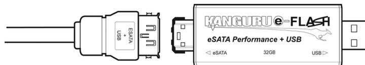
3. After the eFlash has been connected via eSATA, connect it to a USB port. You can use a USB extension cable (not included) to connect via USB, or if you used an eSATA extension cable you can connect the eFlash directly to a USB port.
