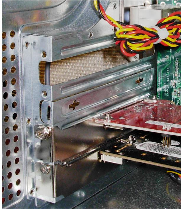
10. Insert the Power Over eSATA bracket into the open PCI bay and fasten it in place using the screw provided.
