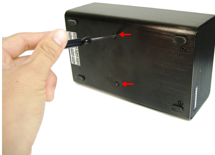
figure 1: Removing the bottom screws
