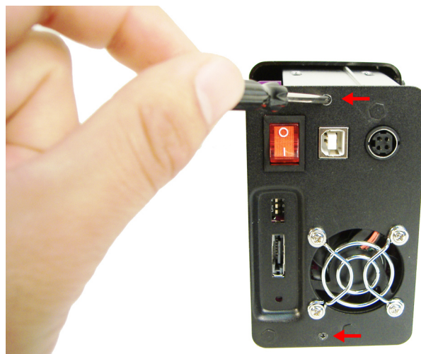
figure 3: Removing the Backplate screws
