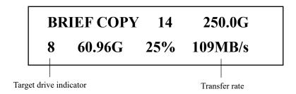
The Target Drive Indicator will inform you which drive is currently selected. The Transfer Rate will show you the speed of this drive. **Note:** The transfer rate information is not static and can fluctuate, sometimes significantly.
