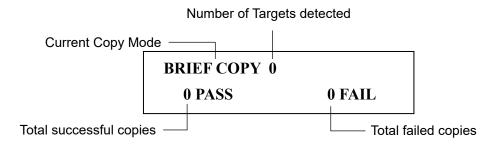
**Note:** The system will not detect any connected drives before the duplication starts. Therefore the "Number of Targets detected" value will remain zero until you execute the copy process.
