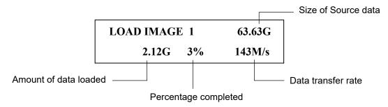
6. When the load process has completed you can remove the Master HDD.
