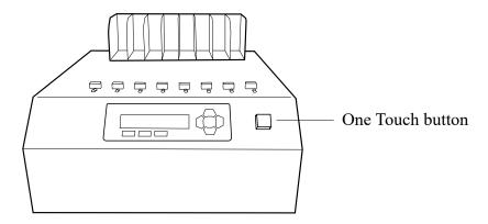
The One Touch button simplifies operations by allowing you to press one buttong to start and clear jobs. The button's color changes depending on the duplicator's status:
